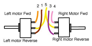
Wiring for SPDT Momentary Toggle Switches
